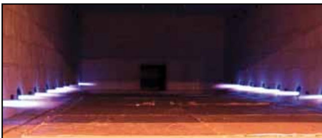
Rekuperatorbrenner an einem Herdwagenofen Recuperative burner on a bogie hearth furnace by courtesy of ARES Industrial Furnace Co., Ltd.
