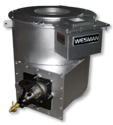
The burner fires tangentially inside the shell lining into a circular combustion space so that the hot gases surround the crucible to ensure uniform heating. Waste gases exit through a flue at one side, allowing comfortable working conditions for the operator. Normally the flue discharge is upward for top exhaust. Optionally, waste gases can be collected in a fume extraction hood for discharge outside production area.
