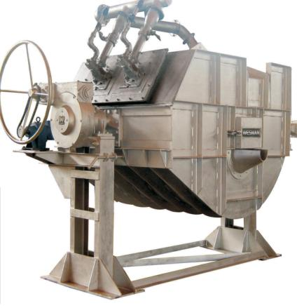
The furnace is provided with a tilting gear arrangement on one side shaft extension comprising a worm, worm wheel, bevel gears and large hand wheel for easy manual operation. A motorized drive arrangement with inching facility is also available as an option.
